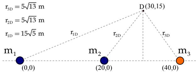
$$V_D = -G \frac{m_1}{r_{1D}} - G \frac{m_2}{r_{2D}} - G \frac{m_3}{r_{3D}} = -6,67 \cdot 10^{-11} \left( \frac{10}{15\sqrt{5}} + \frac{10}{5\sqrt{13}} + \frac{50}{5\sqrt{13}} \right) \Rightarrow$$
