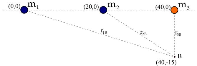
$$V_B = V_1 + V_2 + V_3 = -G \frac{m_1}{r_{1B}} - G \frac{m_2}{r_{2B}} - G \frac{m_3}{r_{3B}}$$
